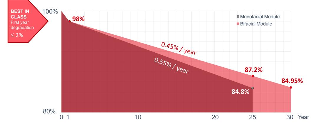
LID (Light Induced Degradation) refers to the initial degradation that all Crystalline PV modules suffer when first contact with light, this phenomenon is intrinsic to the photoelectric effect.
